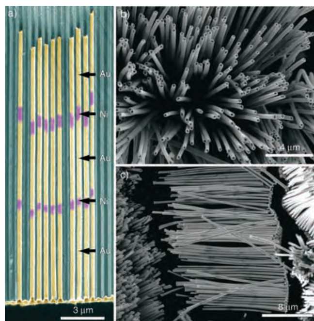
Figure 3. SEM images of multisegmented metal nanotubes with a stacking configuration of Au-Ni-Au-Ni-Au along the nanotube axis. a) Cross-sectional SEM image of as-prepared metal nanotube-AAO composite, which shows metal nanotubes embedded in an alumina matrix. The signals from Au and Ni are shown in yellow and purple, respectively. b) and c) SEM images of multisegmented metal nanotubes after removal of alumina matrix with NaOH (1.0 M); part c) clearly shows the stacking configuration of multisegmented metal nanotubes in which the segments with bright and dark image contrasts correspond to Au and Ni, respectively.
